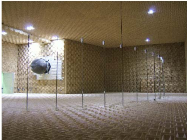
(a) Fan rig installed in anechoic chamber
