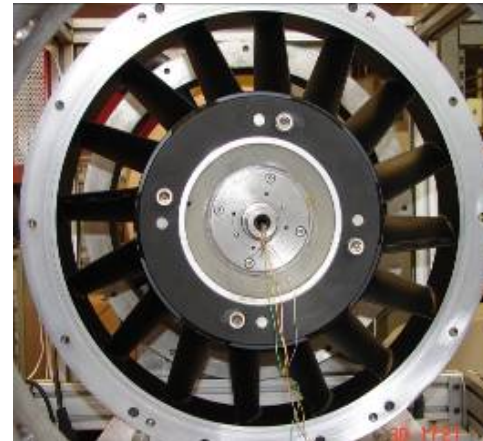
16-vane stator
